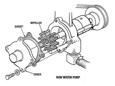
**CAUTION:** If any of the vanes have broken off the impeller, they must be found to prevent blockage in the cooling circuit. They often can be found in the heat exchanger.
