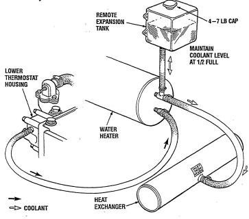
WATER HEATER LOCATED ABOVE THE ENGINE
