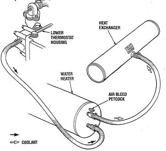
WATER HEATER LOCATED BELOW THE ENGINE
