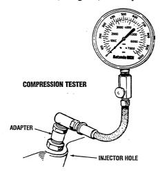
If a weak cylinder is flanked by healthy cylinders, the problem is either valve- or piston-related. Check the valve clearances for the weak cylinder, adjust as needed, and test again. If the cylinder is still low, apply a small amount of oil into the cylinder to seal the rings, and repeat the test. If the compression comes up, the rings are faulty.
