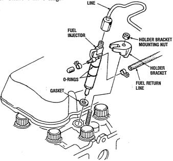
**REMOVING THE FUEL INJECTORS**
