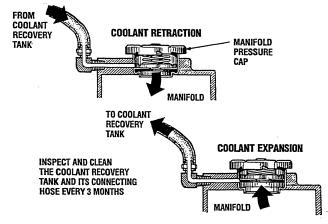
**NOTE:** Periodically check the condition of the manifold pressure cap. Ensure that the upper and lower rubber seals are in good condition and check that the vacuum valve opens and closes tightly. Carry a spare cap.
