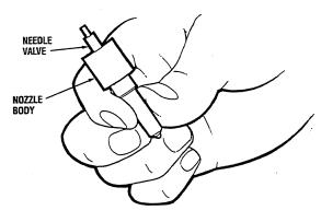
CHECKING THE NOZZLE BODY AND NEEDLE VALVE
