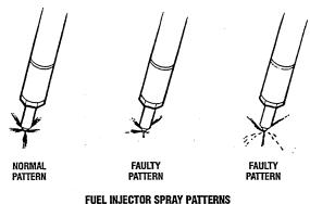
Normal Pattern: The fuel is sprayed uniformly and finely from all five injection nozzle holes.
