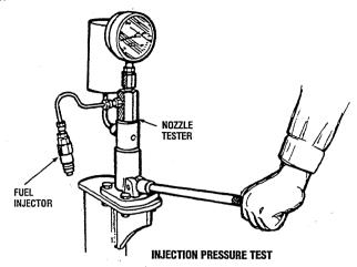
6. If the injection starting pressure is not within the specified range, adjust it by replacing the shim with one of a more appropriate thickness.
